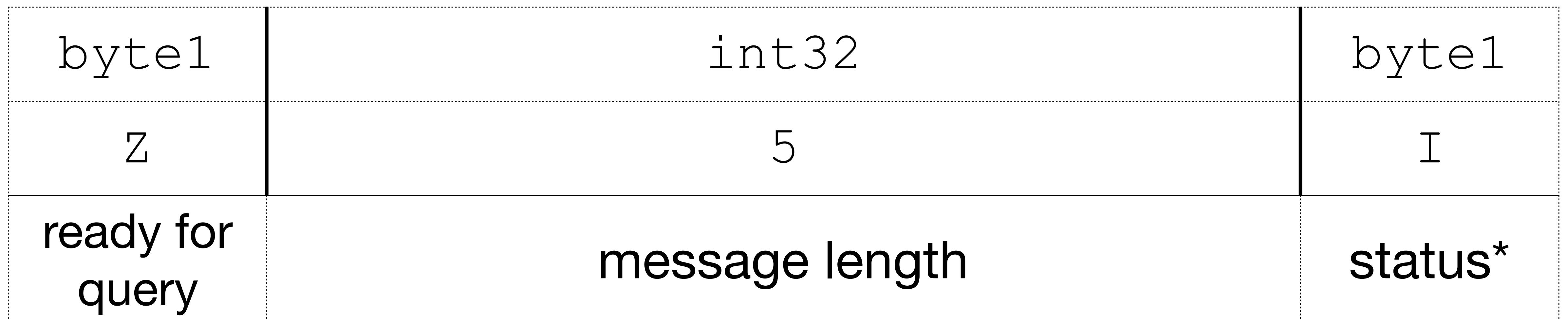
\* – I: idle (not in a tx block), T: idle (in tx block), E: failed tx block
